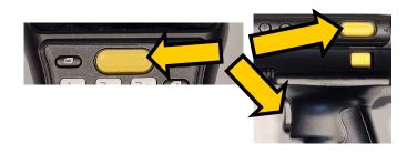
There are multiple buttons that can be pushed to scan a barcode: the trigger on the pistol attachment, the yellow button just below the screen, and the yellow buttons on either side of the device.
