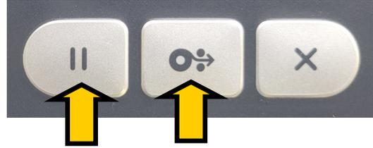
While holding these buttons down, turn on the printer. Continue holding the Pause and Feed buttons until the Status indicator is the only light lit. Release the two buttons and wait for the Status indicator to turn green. Some labels may be fed through the printer when this process is complete.
